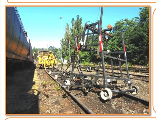
A derailed Projector Buggy, unnoticed by the operator, is a common cause of mounting costs in rail maintenance:
