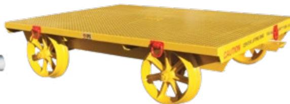
Push cart complete with steel deck. 10,000 pounds capacity with four 16" wheels. Deck measures 67" wide x 85" long; 96" overall cart length, and 20" deck height (above rail). Also available in 10" wheel model.
