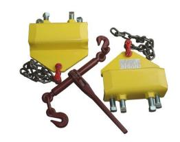
**Description:** Three-part device designed to pull rails back into alignment (such as after a derailment) so that re-railing can proceed. Specially designed 1/2" thick steel, formed plate rail-pull clamps allow cars to pass over the clamps without damage at slow speeds.
