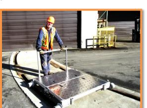
**Description:** This collapsible aluminum rail buggy boasts a 5,000 lbs. capacity. 50" long x 63-1/2" wide, it runs on 5" diameter insulated aluminum wheels for 56-1/2" gauge rail. The cart can be moved from either end with the moveable push rail and the entire assembly folds up for efficient storage and transport. Parking brakes at both ends provide safety during loading and unloading.
