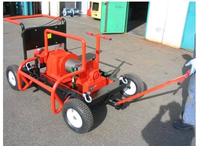
**Description:** The IPS Locomotive Winch Cart is an effective way to pull locomotives in for service and maintenance on level or near level track. The heavy-duty, 3 phase electric hauling winch is mounted on pneumatic wheels, and solid transport frame. This cart is supplied complete with electrical box and power cord, 250' of ½" diameter wire rope with attachment hook, locking anchor pin, floor anchor plate, tow handle, and jacking system.
